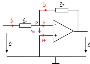
$$H(j\omega) = \frac{v_2}{v_1} = -\frac{Z_2}{Z_1} \text{ et } Z_{IN} = Z_1$$
