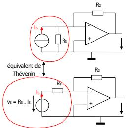
$$v_2 = -R_s \cdot I_s \cdot \frac{R_2}{R_s} = -R_2 \cdot I_s$$
