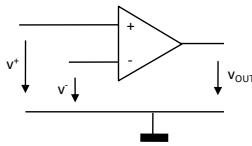
$$v_{\text{out}} = A(v^+ - v^-)$$
