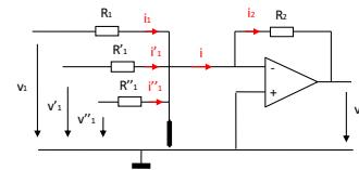
$$i_1 = \frac{v_1}{R_1}, i'_1 = \frac{v'_1}{R'_1}, i''_1 = \frac{v''_1}{R''_1} \quad v_2 = -R_2 \cdot I_2 = -R_2 \cdot I$$
