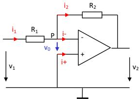
$$v_{\text{out}} = A(v^+ - v^-)$$
