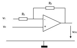
$$V_{OUT} = V_2 \cdot \frac{R_1 + R_2}{R_1} - V_1 \cdot \frac{R_2}{R_1}$$
